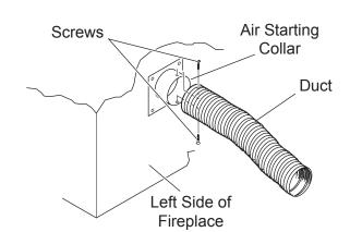
Figure 21 - Attaching Outside Duct to Starting Collar
